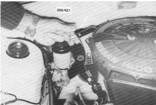
Checking for vacuum at the servo unit. The engine must be running for this test.
