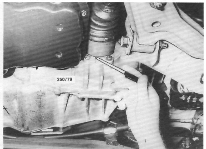
Check the drive shaft oil seals as a likely leak source.
