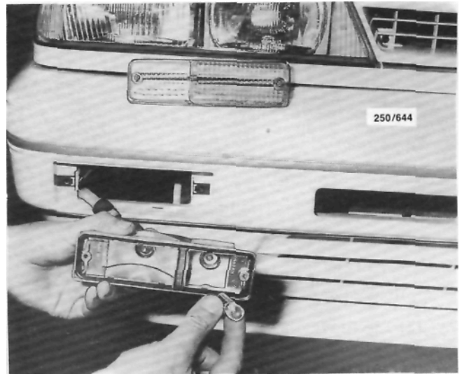
Renewing the front combination lamp bulb. Pulsar models.
