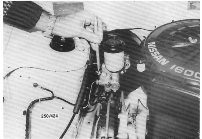
Check the brake pipe unions for leaks.
