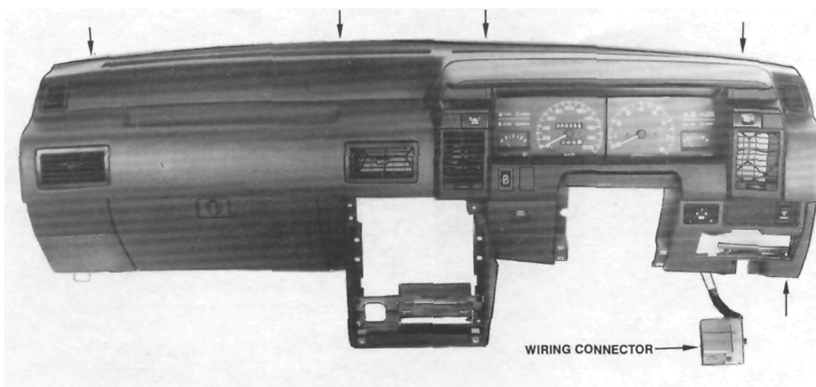
View of the dashboard removed from the vehicle. The arrows indicate the location of the retaining bolts.
