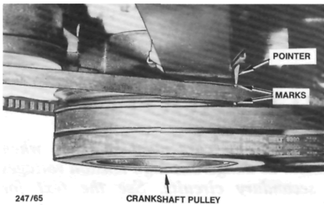
View of the engine timing marks showing the 10 deg BTDC crankshaft notch aligned with the pointer on the front of the engine.
