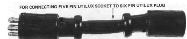
Useful connections which can be used if the trailer to be towed is fitted with different type plug to the towing vehicle socket
