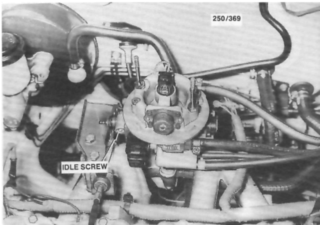
Installed view of the throttle body assembly showing the location of the base idle adjusting screw. 1.6 liter engine.
