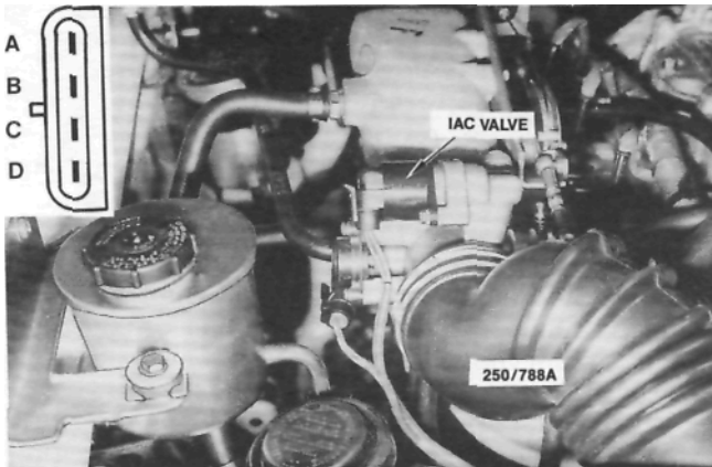
Location of the idle air control (IAC) valve. Inset shows the terminal identification.
