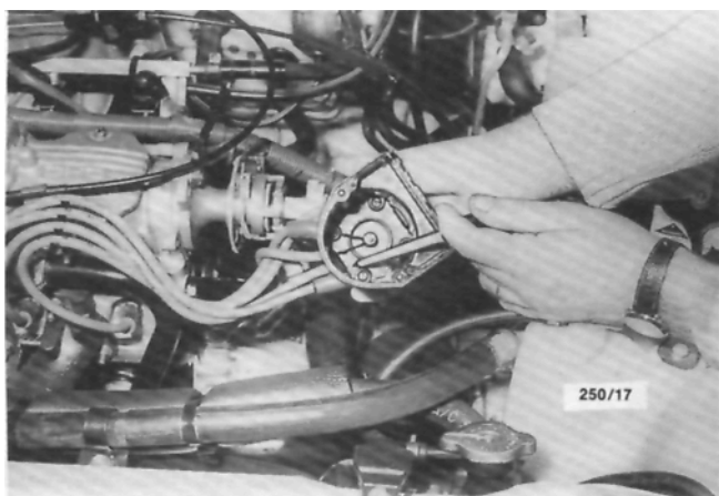
Check the distributor cap for cracks or tracking between the terminals.
